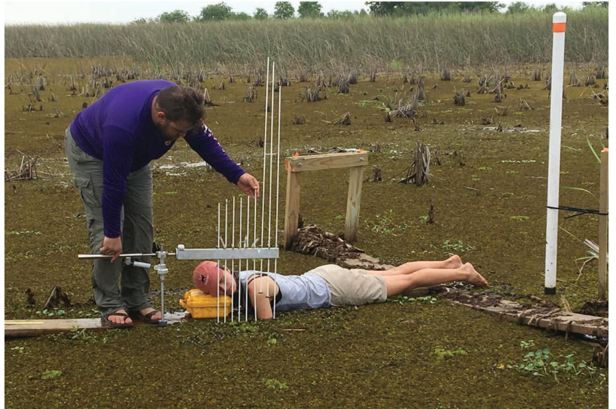
Ashley Booth and Clay Tucker taking readings at a surface-elevation table at J.D. Murphree WMA. (Credit Alex Freeman)
