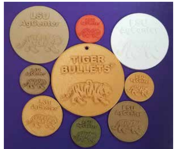
These prototype wood fiber-filled, recyclable and biodegradable coins were made in Wu's lab.
