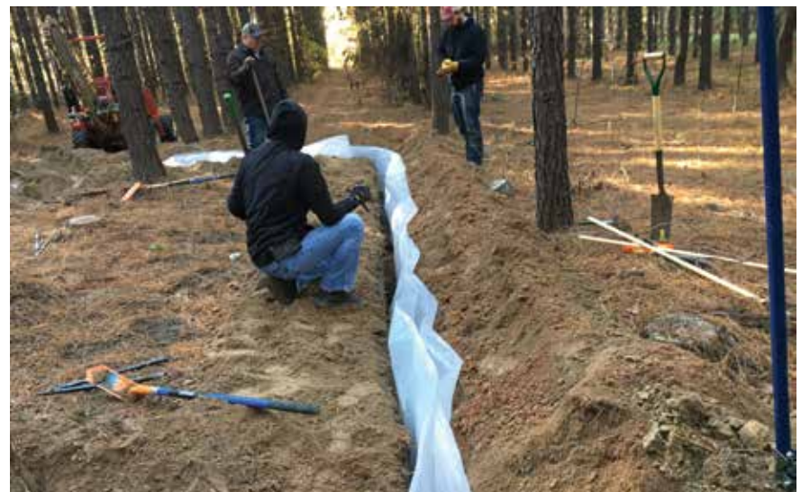
Plastic sheeting was installed within the trenches around the research plots to block the flow of water through the soil. In the months ahead shelters will be constructed over the soil in the drought treatments to block rainfall for this experiment.
