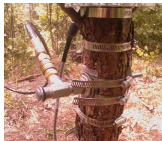
Figure 1. Injecting air into the stem of a young loblolly pine tree to reduce water flow through the stem.
