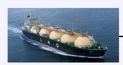
**Shipping:** The typical LNG carrier can transport125,000 to 138,000 cubic meters of LNG, which will provide about 2.6 to 2.8 bcf of natural gas. The typical carrier measures 900 feet in length, 140 feet in width and 36 feet in water draft, and costs about \$160 million.
