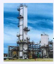
**Liquefaction:** Gas from the production field comes to the liquefaction plant. Contaminants are removed and the gas is cooled to a temperature of -256°F. By liquefying the gas, its volume is reduced by a factor of 600.
